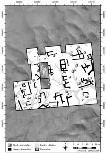
Fig. 8: preliminary results of geomagnetic survey in Area 33 at Shahr-i Sokhta.
